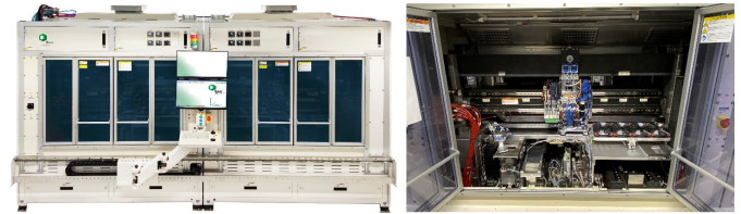
Figure 5. Dual TC bonder exterior (left) and interior showing inert tunnel, bondhead, auto tool change etc
